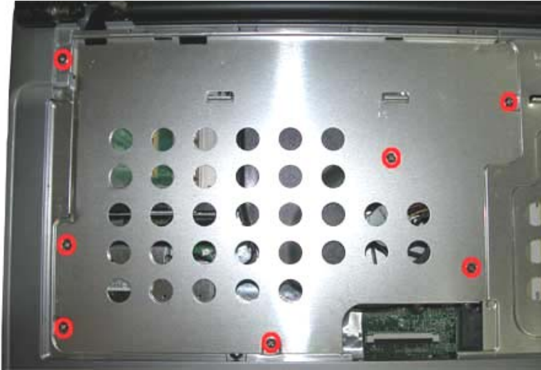
Fig. 12 Removing the screws retaining the Heat Plate
